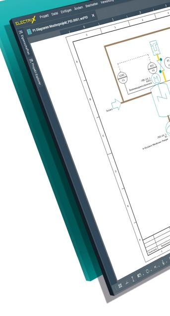
Piping and Instrumentaion diagrams are created using the PI discipline. P&ID drawings already in DXF or DWG format can be read in no time. The intelligent linking of measuring points and devices to schematic diagrams and other disciplines enables their interaction to be presented logically and linked to the automation technology design.
